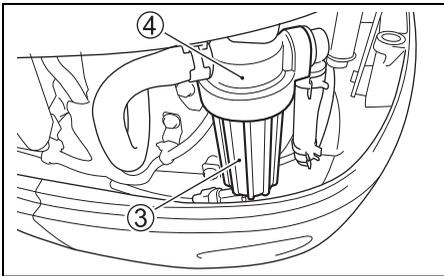
7. Drain the fuel and water in the filter cup into a suitable container.
