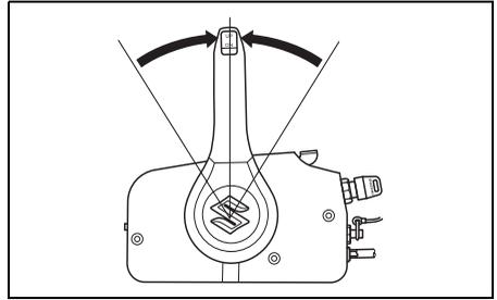
6. Make sure the lock plate is in place and attach the emergency stop switch cord to a part of your body.
