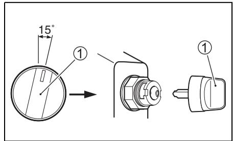
2. Insert the emergency key ② into the key cylinder.
