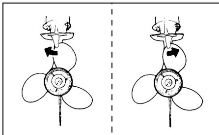
3. Tighten the bolt that holds the trim tab in place.
