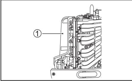
2. Remove the bolt securing the ignition coil.
