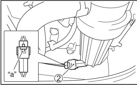
5. Place a rag under the filter before removal to catch any spilled fuel.
