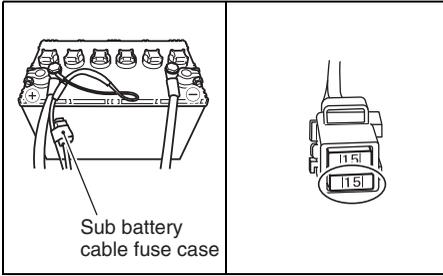
5. Inspect the fuse and replace with new fuse if needed.
