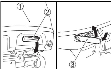
2. Pull out the oil dipstick and wipe oil off with a clean cloth.
