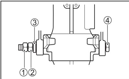
4. Reposition the tilt pin in the desired holes.
