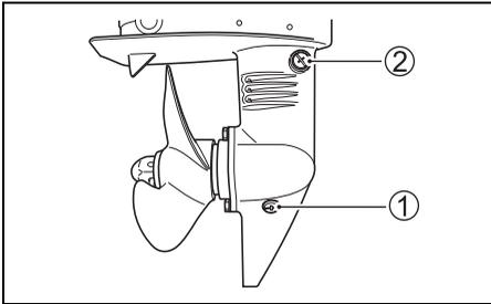
3. After the oil has drained completely, inject the specified gear oil into the lower drain hole until it just starts to come out of the upper hole. Approximately 0.07 L (0.07/0.06 US/Imp. qt.) of oil will be required.
