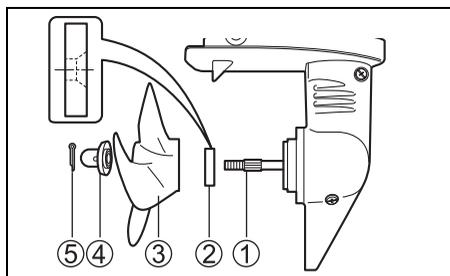
To remove the propeller, reverse the above procedure.
