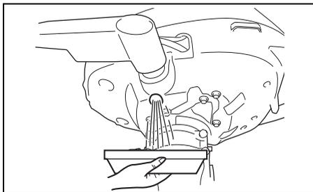
5. After draining, secure the engine oil drain plug with a new gasket.
