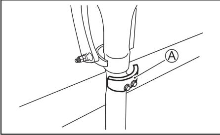
3. Turn the fuel cock lever to the right (off position) and tighten the air vent screw on the fuel filler cap.
