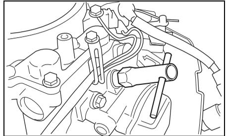
To maintain a strong spark, you should clean and adjust the plug at the intervals shown in the maintenance chart. Remove carbon deposits from the spark plug using a small wire brush or spark plug cleaner, and adjust the gap according to the following chart:
