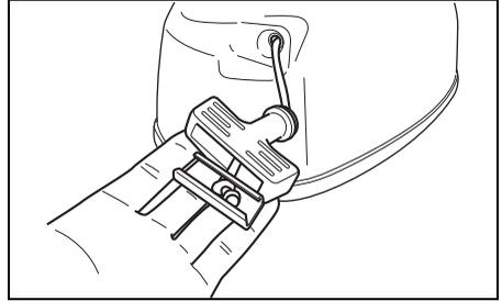
5. Install the starter grip holder to the end of rope.
