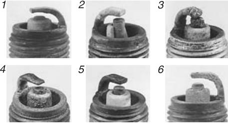
1. Excessive wear    2. Breakage    3. Melting
