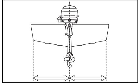
After installing the motor, check to make sure that steering and tilt movement are not obstructed by any part of the boat.
