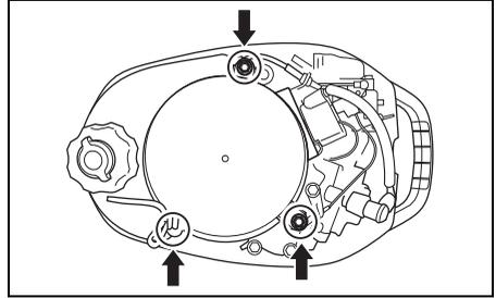
4. Lift off the recoil starter assembly. Re-tighten the fuel tank by using the recoil starter bolts removed.
